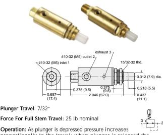
**Operation:** As plunger is depressed pressure increases proportionally to the travel; when plunger is released the input is closed and the output pressure is exhausted to atmosphere
